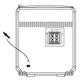
**<u>AM</u>**: The AM bar antenna is inside the cabinet of the main unit. You may need to change the position of the main unit until you find the position that provides the best reception for your favorite AM stations.
